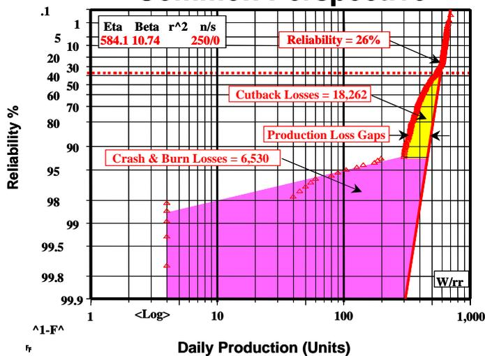
**Figure 1: Example Of A Troubled Processes**
