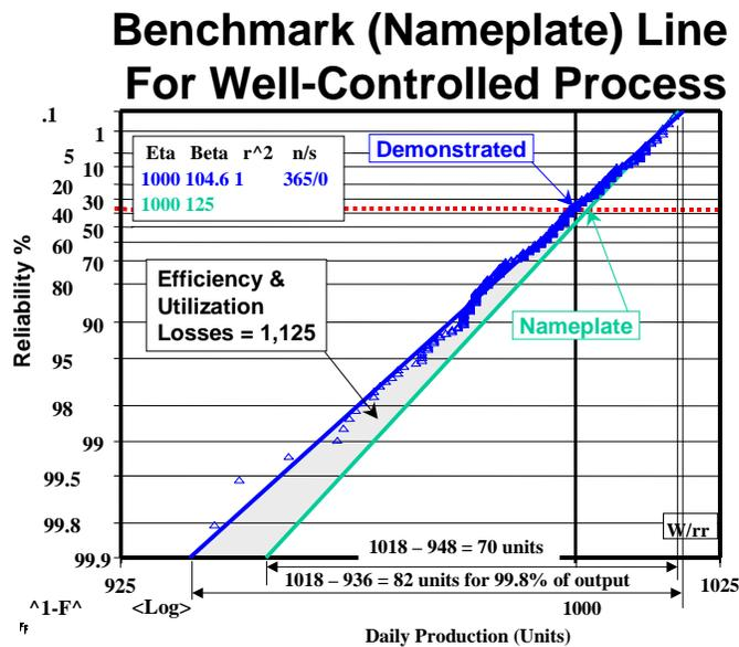
**Figure 5: Benchmark With Losses Identified**
