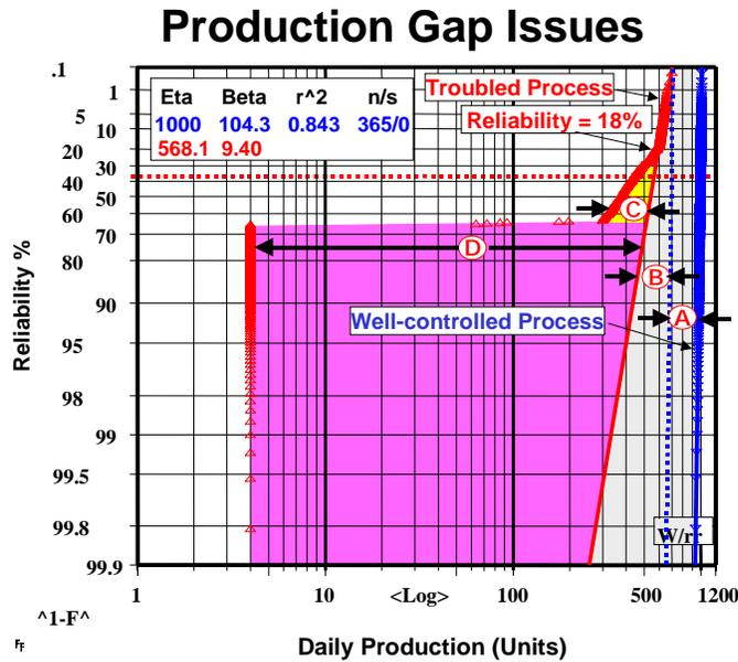
**Figure 4: Production Gaps Between Two Processes**
