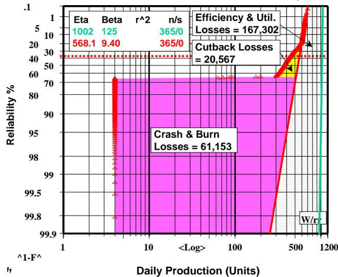
**Figure 6: Troubled Process With All Losses Identified** regarding utilization issues.
